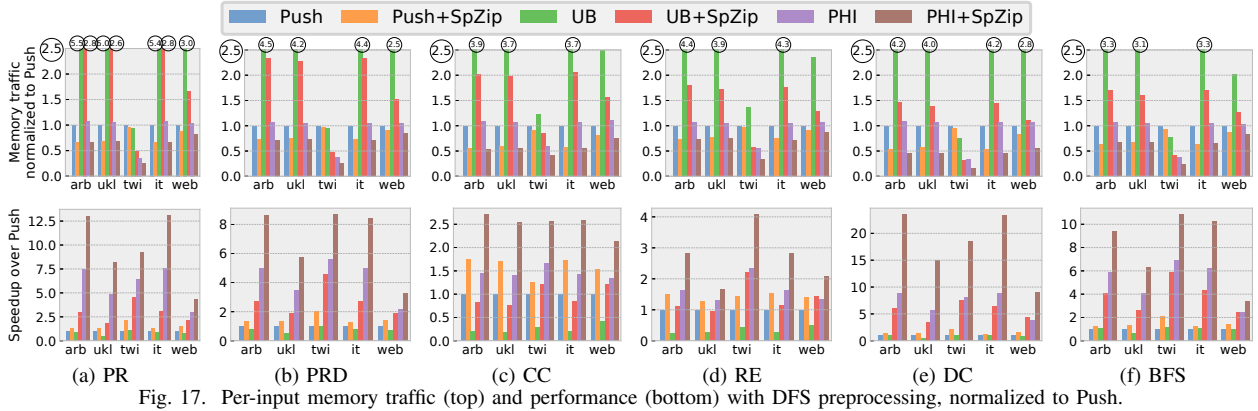
Fig. 17. Per-input memory traffic (top) and performance (bottom) with DFS preprocessing, normalized to Push.
